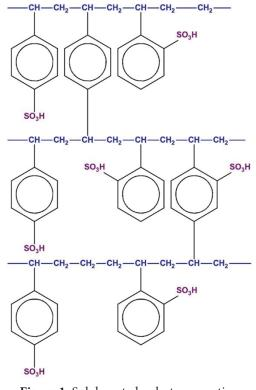
Figure 1: Sulphonated polystyrene cation exchange resin.
